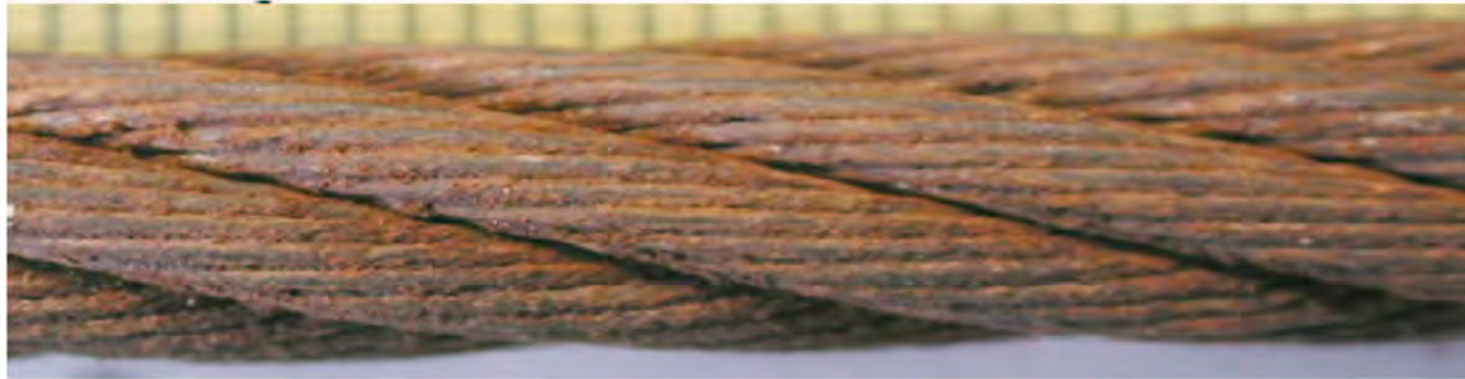
Figure I.1 — Beginning of surface oxidation – staining of the outer wires Rating: 20% towards discard
